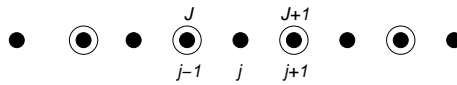
Figure 14: Illustration of coarse and fine meshes in one dimension for the purpose of linear interpolation (prolongation), of coarse grid values to the fine grid. Refer to the text for details.
